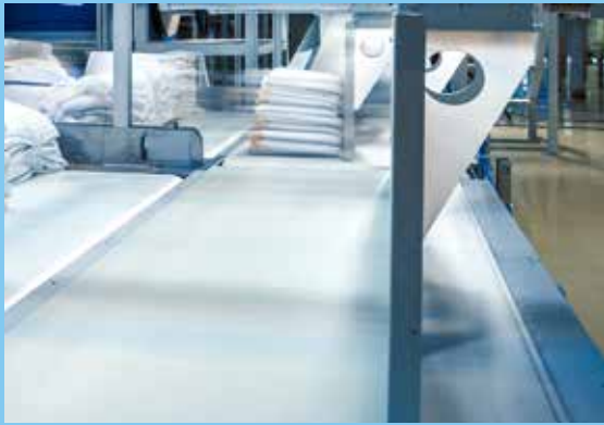
Sideway Pusher for fully automatic and flexible stack sorting
