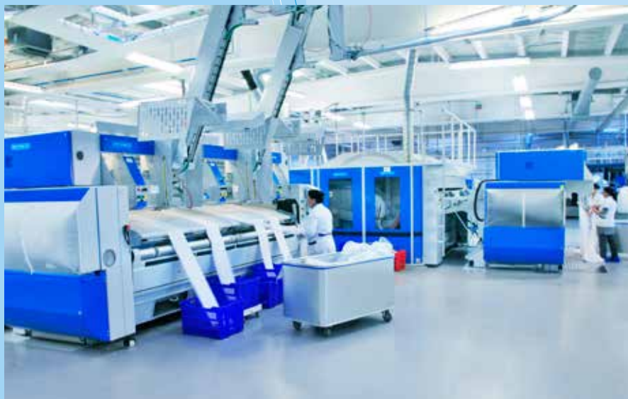
Optional pivotable deloading stations of the Jenrail 2000 Automatic system allow small-piece feeding into the Jenfeed Logic Plus Automatic
