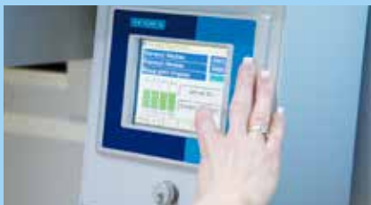
Control centre of the Jenrail 2000 Automatic system with Jentrol HMI PLC and touch screen.
