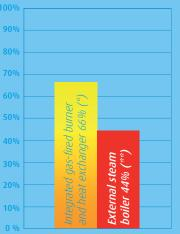
Energy efficiency of direct heating vs external steam boiler
