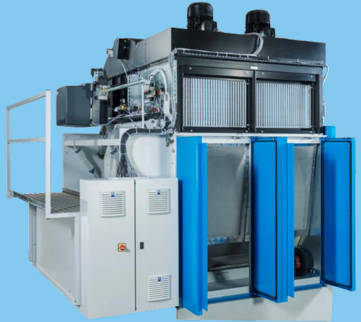
WR 120 with integrated, easily accessible heat exchangers
